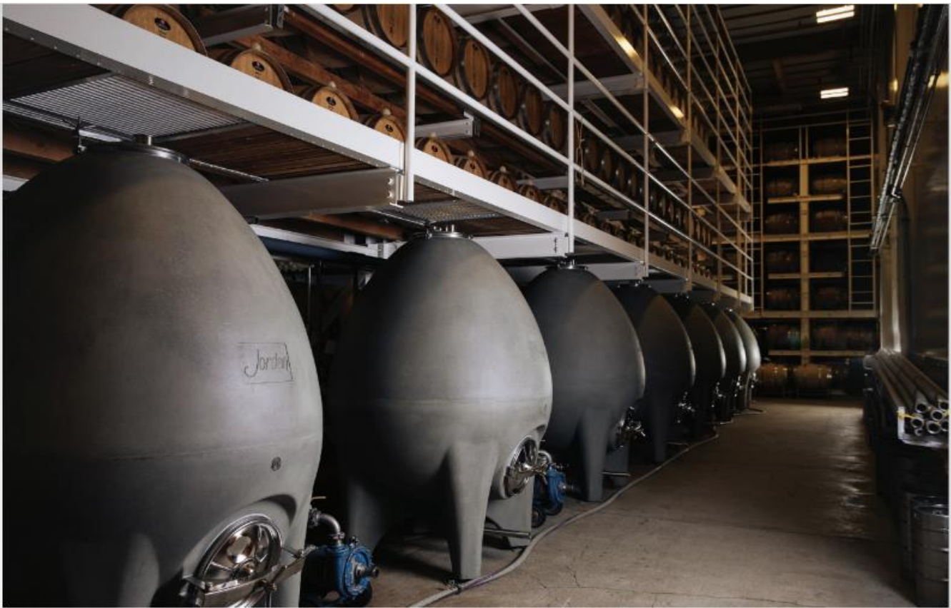
The Jordan cellar houses eight concrete eggs.
